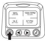
When the PowerView receives a fault code from an engine control unit the single or four parameter screen will be replaced with the "Active Fault Codes" message.
